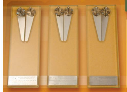
The CF-150B cell fusion instrument operates with specially designed high precision electrode chambers. The chambers are made with three different gap distances; 250µm, 500µm and 1000µm with corresponding model names of GSS-250, GSS-500 and GSS-1000, respectively. The electrodes are made of high quality stainless steel and attached to a thick glass slide. All the materials used are biologically friendly, non-toxic. The electrodes can be kept clean and sterile with ethanol.
