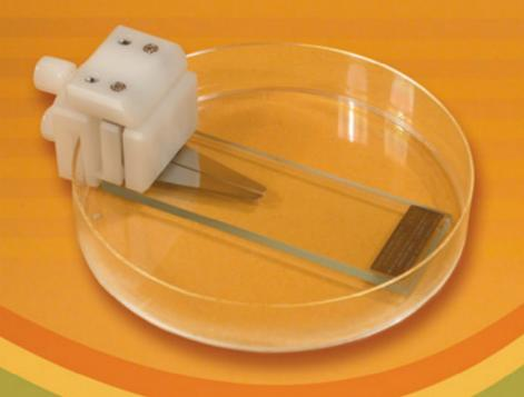
This "quick clip" design secures the electrode to the side of the tissue culture dish (or its lid). It eliminates the risk of accidental sliding during electrofusion, and it provides a permanent attachment for the electrode wires. The clip can be used with any of the three electrodes GSS-250,GSS-500 or GSS-1000.
